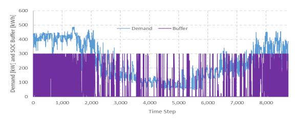
Figure 4: Demand and SOC of thermal buffer storage.
